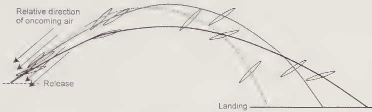
FIG. 15.10 Effect of angle of attack on discus flight distance. The discus with a negative angle of attack (dark line) travels the greatest distance because this orientation maximises lift and decreases drag through the entire trajectory. Throws with a positive angle of attack (lightest line) may 'stall' as the drag force increases significantly in the downward phase of the trajectory.
