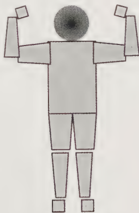
FIG. 7.2 Most objects can be modelled as a series of common geometric shapes. This human is 'built' out of basic shapes of which the radii of gyration can be relatively easily determined.
