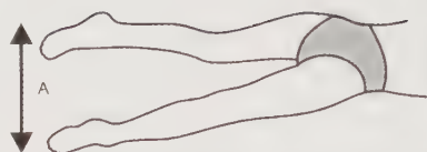
FIG. 14.7 Since form drag is proportional to the frontal cross-sectional area of the swimmer (remember F_d = kAv^2 ; Chapter 14), kicks with greater amplitude ( A ) will increase form drag.
