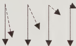
FIG. 1 If an object is falling with gravity, the force of gravity (and acceleration of the object) will always be greatest in the vertical plane. Therefore, the hypotenuse of a right-angled triangle is always drawn vertically (solid arrow). The magnitude of a vector at any angle from vertical will always be less, with the magnitude decreasing with increasing angle (dashed arrows).
