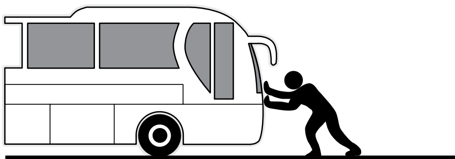
FIG. 5.2 A large bus moving quickly has a large momentum. It would take a large force produced over a significant time period to stop it.
